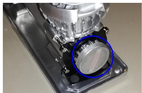
The ambient air should be as pure as possible. Absolutely avoid the proximity of an engine exhaust, smoke and suspicious odors. Preferably inflate in the open air or in a ventilated place. If the intake air is of good quality, the air contained in **EAZYDIVE** will be of good quality and will easily check the standard in this matter: European Standard EN 12021. The compressor is not lubricated with oil, so there is **NO trace of oil** in the air breathed.
