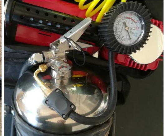
Inflation by a single tire valve on the scuba tank
